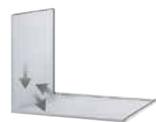
Cabinets constructed with 18mm board and 1mm edging
